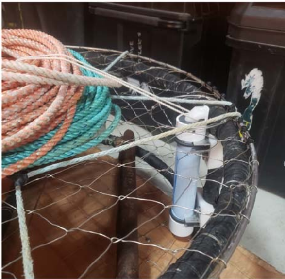
Vertical installation on a crab trap with the TR4RT inside the trap with line retainer.
