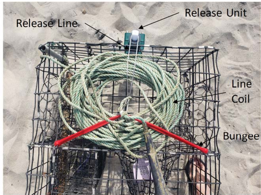
Rigging setup on a lobster trap.
