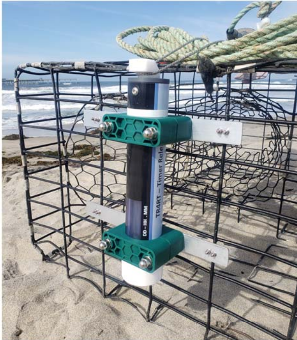
Vertical installation on a lobster trap with the TR4RT outside the trap and no line retainer.
